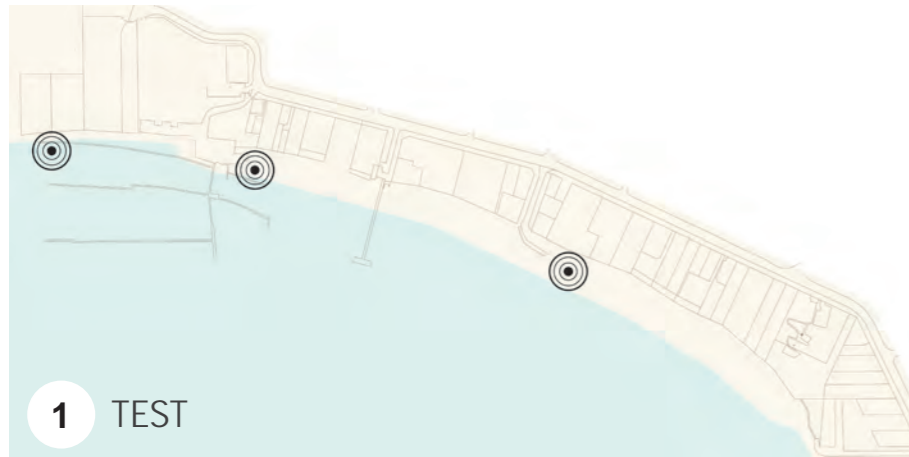
1 TEST Ground penetrating radar with vacuum extraction and geotechnical assessment of rubble at Chester Road. Testing of sediment at CYC. Requires cultural monitoring.
